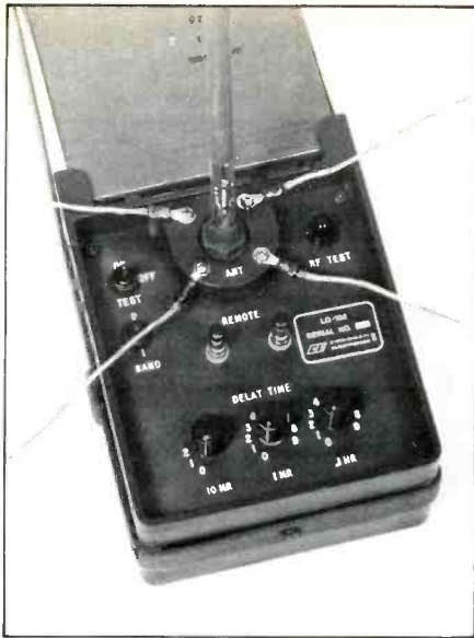
The LQ-102 is a small jammer which operates between 30 and 76 MHz. It is made solely for the military and is not available commercially. (Photo courtesy Cincinnati Electronics Corp.)
