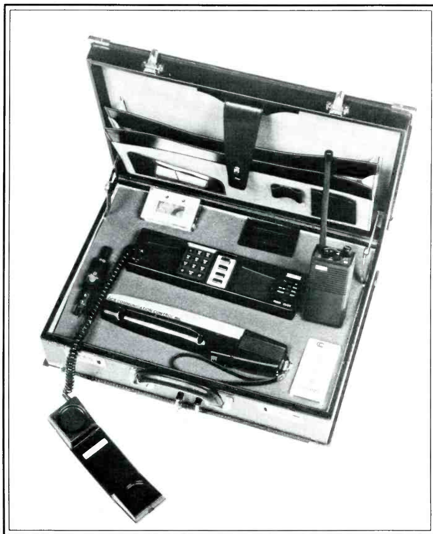
This portable security communications suitcase is produced by CCS Communications Control, Inc. It includes a sophisticated voice scrambler.
