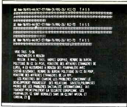
Figure 5: An RY test slip that is followed by a French transmission.
