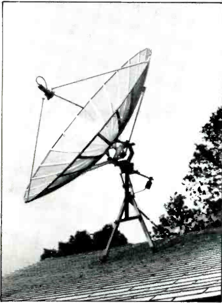
Mounted on a roof is a 10 foot wire mesh dish. (Photo courtesy of Microsat)
